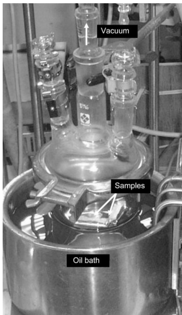
Figure 1 Photograph of conversion experiment. Samples show selective reflection characteristic of cholesteric liquid crystal.
